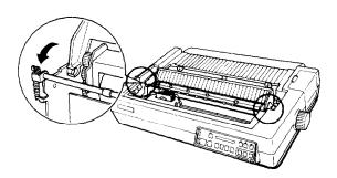
3. Remove the paper eject guide by tilting it forward, then lifting it up and off.
